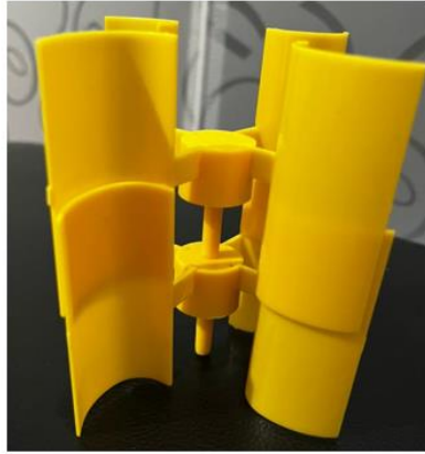
(a) Turbine assembly using glue
