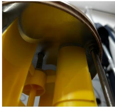
(c) (d) Bolt and nut used to tie rod and tin top and bottom tin case
