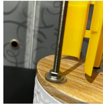
(c) (d) Bolt and nut used to tie rod and tin top and bottom tin case
