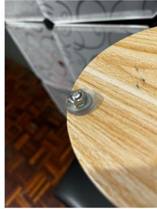
(b) Silicone washer are used to seal gap
