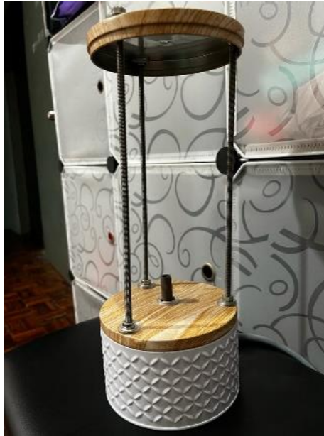
Figure 3.7 Casing Tin and Metal Rod for Casing Structure
