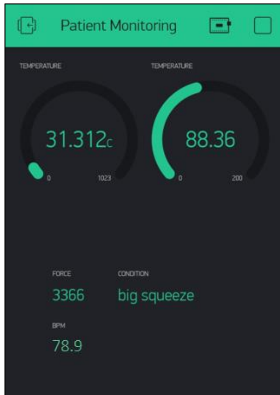
Figure 4.25: Data collecting of sensors in patient monitoring system IoT
