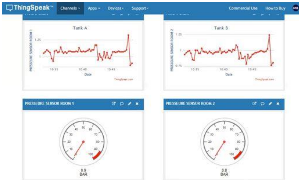
Figure 4.9 Pressure sensor detection gas leakage in tanks results in ThingSpeak
