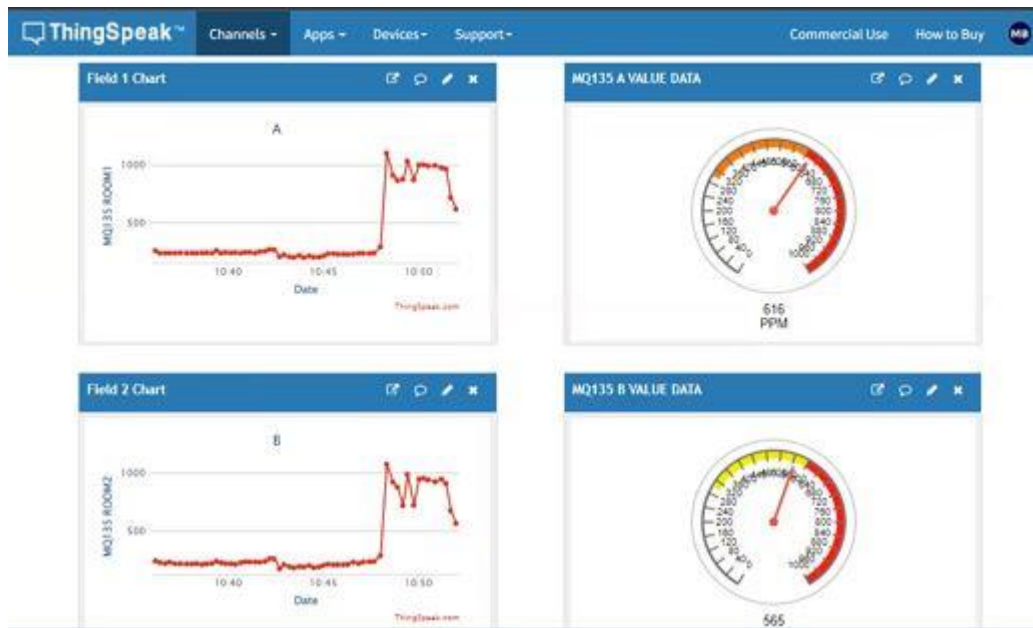
Figure 4.11 Gas sensor before detecting any leaks in ThingSpeak
