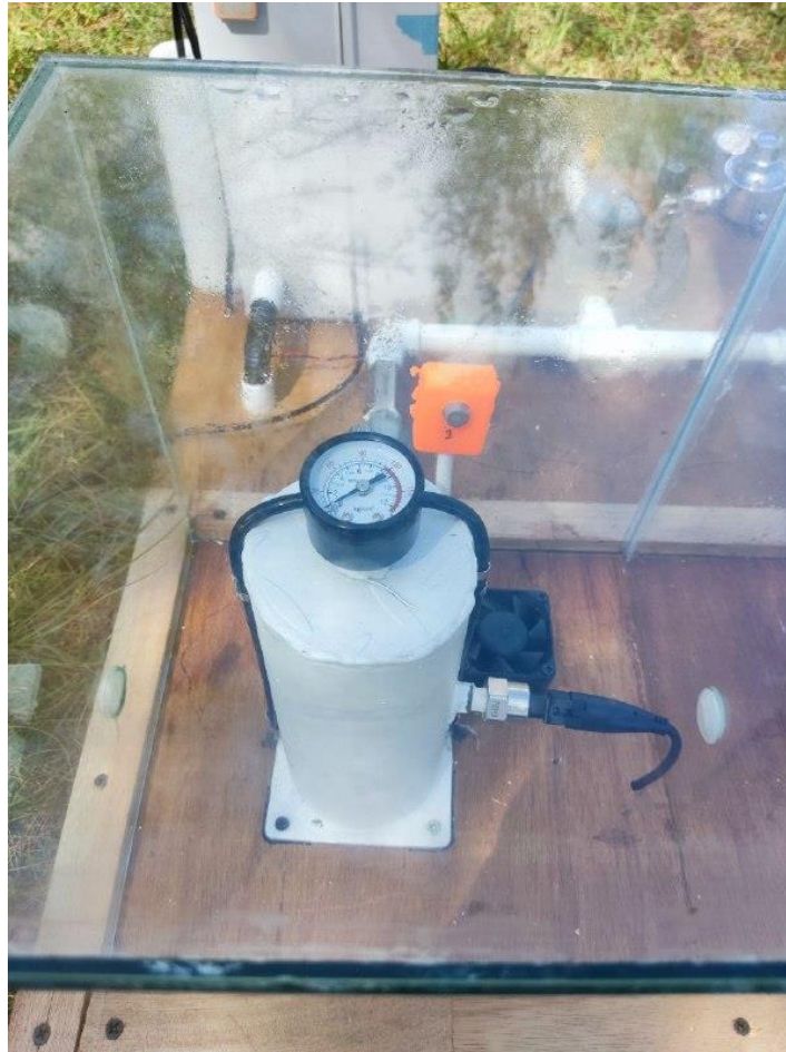
Figure 4.3 In storage room also will be put ventilation fan and MQ135.
