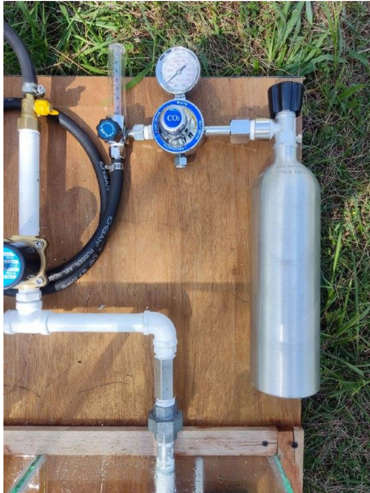
Figure 4.5 The gas regulator for reduce the pressure of gas from 1000psi to 100psi
