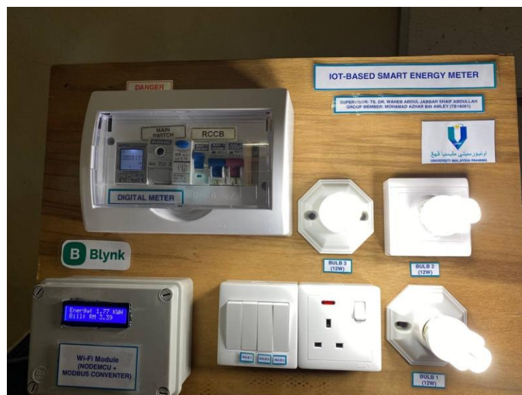
Figure 3.16 Testing and validation with 3 bulbs
