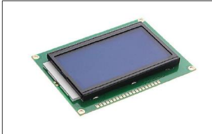
Figure 2.18 ST7920 Graphic LCD
