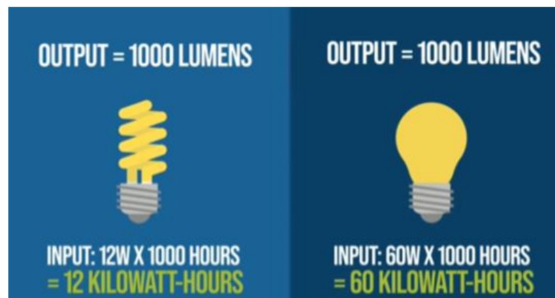
Figure 3.2 Comparison between energy efficiency with bulb
