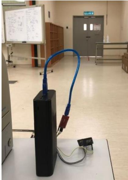
Figure 3.25: Testing of ESP-CAM connected with Power Bank
