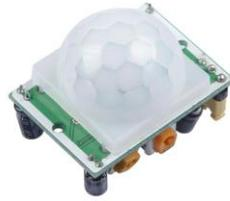
Figure 3.6: PIR Motion Sensor
