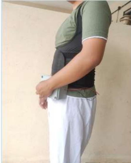
Figure 20: The user is holding the control box and flex sensor is placed on the back of the user.
