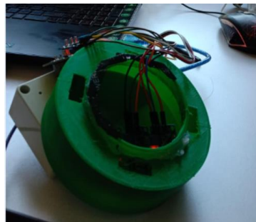
Figure 4.2: Gas Sensor Placement Mechanism tested on Open Air Environment.
