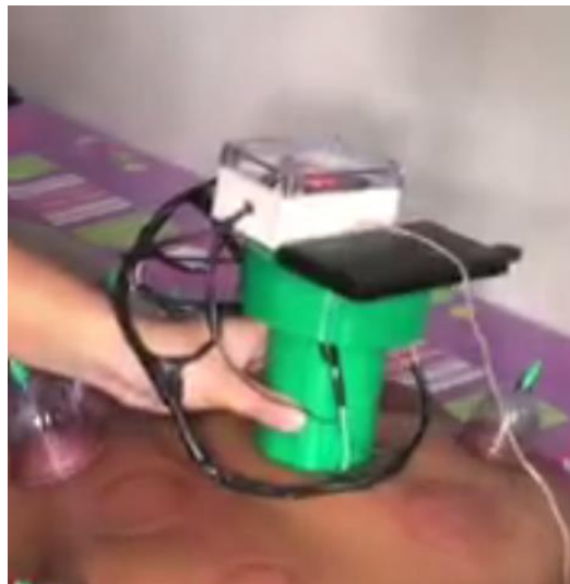
Figure 4.12: Gas Chamber placed on the patient to get reading of gas.
