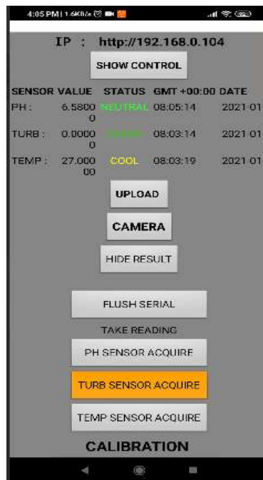
Figure 4.6 Turbidity sensor acquire
