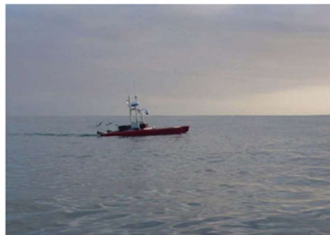
Figure 2.6 ROAZ II Autonomous Surface Vehicle.
