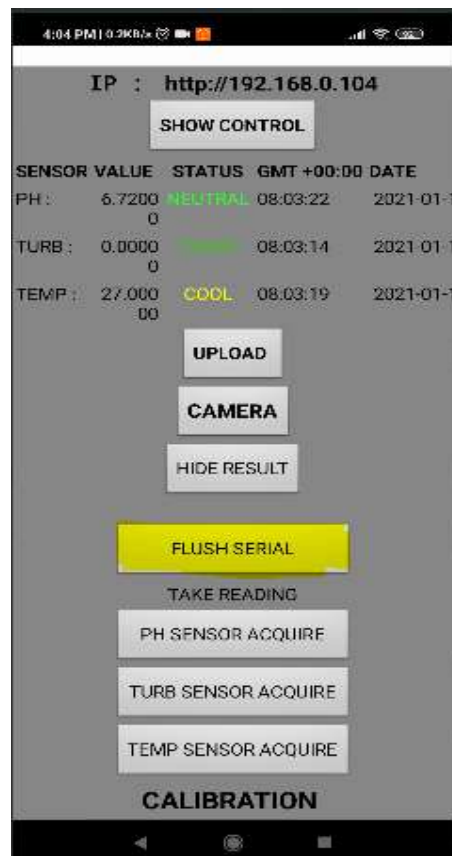
Figure 4.10 Flush function on application
