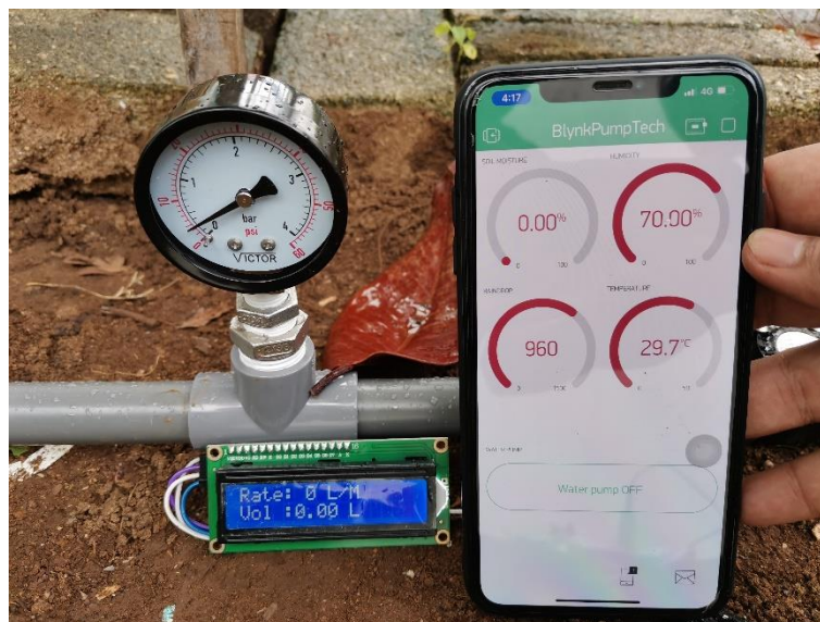
Figure 4.12 Before solenoid valve is ON
