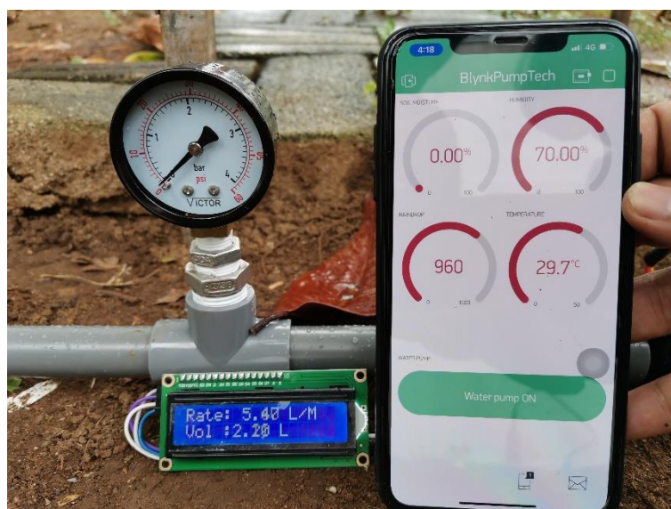
Figure 4.13 After solenoid valve is ON
