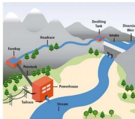
Figure 1.1.2 Run-of-River Hydropower Plant (Diversion) [3]
