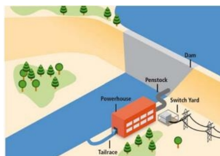
Figure 1.1.1 Impoundment Hydropower Plant (Storage Hydropower Plant) [3]
