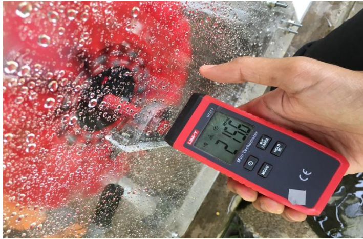
Figure A1 : Measurement for Turbine speed
