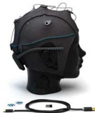
Figure 3. EEG signal measuring Unicorn Hybrid Black EEG Device [13]
