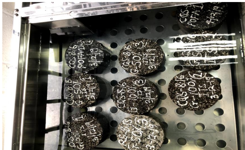
Figure 2. Moisture-conditioned samples in water bath at 60 °C.
