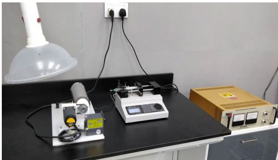
Figure 1. A needle electrospinning setup was used in this experiment
