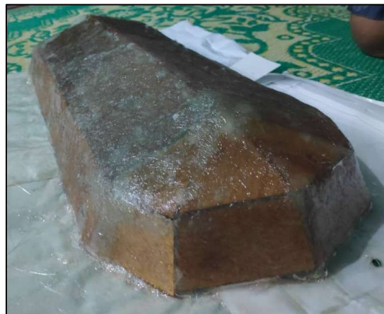
Figure 3.42: Fabrication process of the boat using resin and fiberglass
