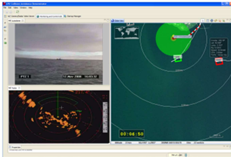
Figure 2.5: Target detected and leaving closest approach zone
