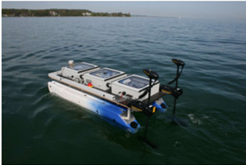
Figure 2.11: USV of the HTWG Konstanz is a twin hull USV for rivers and inland waters
