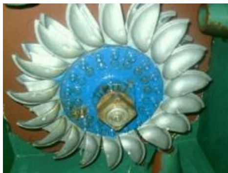
Figure 2.2 Pelton Turbine used in micro-hydro scheme in Bondo, Kenya [37]
