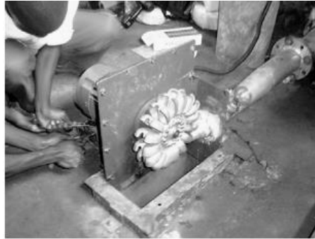
Figure 2.1 Pico-hydro scheme using Pelton Turbine in Kathamba, Kenya [36]
