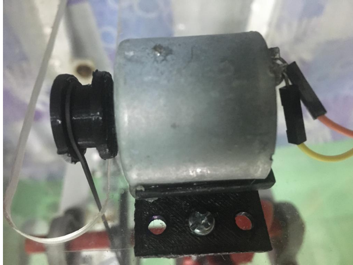
Figure 3.16 PMA motor implemented in prototype as generator
