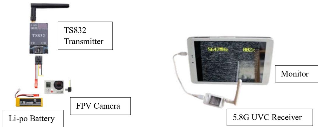
Figure 4.3 Transmitter & Receiver Circuit of Vision System
