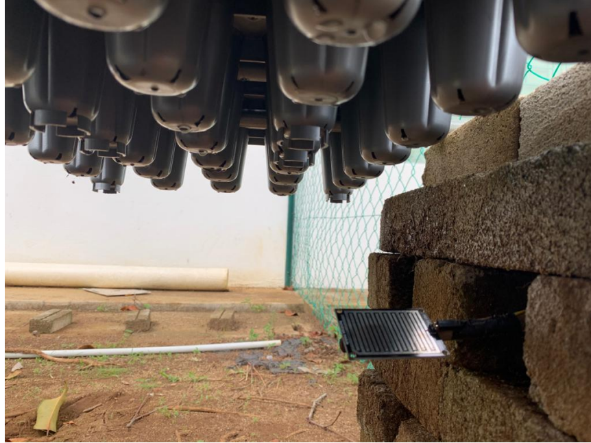
Figure 4.4 Rain sensor setup
