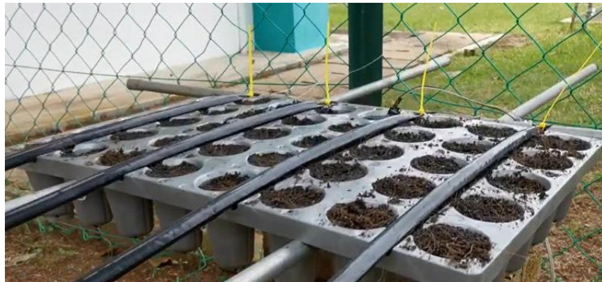
Figure 4.5 Soil moisture setup
