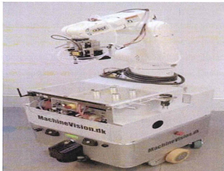
Figure 11: Example of Hybrid autonomous industrial mobile manipulator [8]
