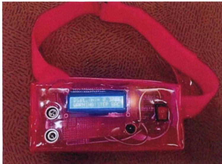
Figure 2.4 Prototype of the ultrasonic sensor system
