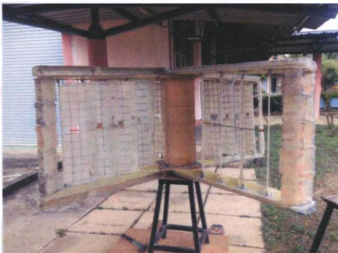
Figure 5 The assembly of one complete new turbine with hinged blade composites (A.N. Johari1*, 2019)
