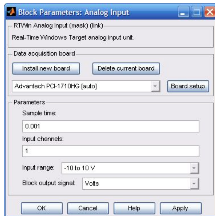
Figure 3.12: Block Parameters of Analog Input
