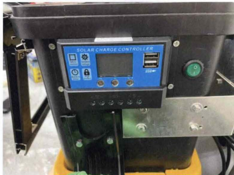
Figure 3-6 Solar charge controller attached with prototype
