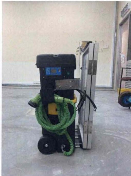
Figure 4-1 Solar panel and solar charge controller attached with prototype
