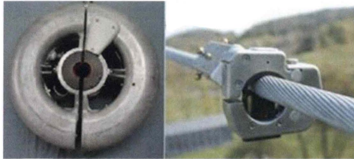
Figure 2.1: Conductor temperature monitors with radio links
