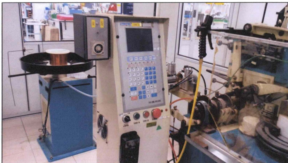
Figure 6.7: CNC Winding Machine with Controller
