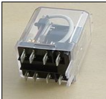
Figure 2.18: A DPDT AC coil relay and symbol of the relay
