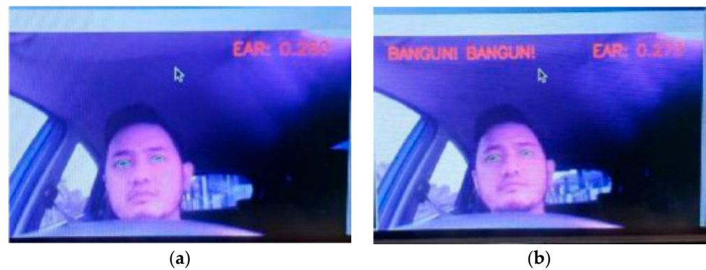
Figure 6. Eye detection. (a) Normal eye state; (b) aspect ratio below threshold.
