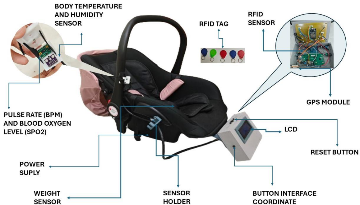
Figure 6. Improvement of the non-invasive monitoring PreeCASE device
