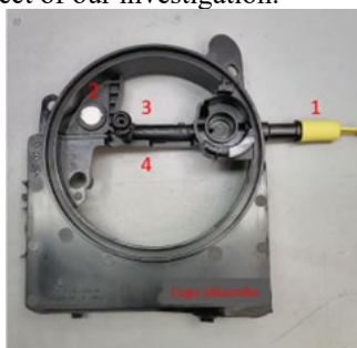
Legend: 1 dust cap, 2 membrane, 3 O-ring, 4 seal retainer
