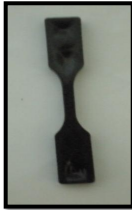
Figure 3.10: Example of PLA/CNT Composite Sample from Injection Molding process
