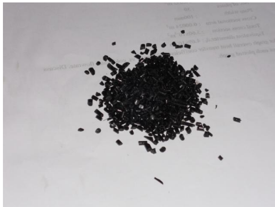
Figure 3.5 : Example of Pellet sample obtain after extrusion process
