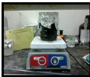
Figure 3.18: Stirring and heating the CNTs
