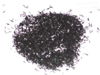
Figure 3.6 : Example of Pellet sample obtain after extrusion process (treated sample)
