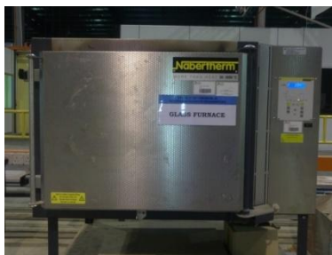
Figure 3.20: Glass Furnace at Universiti Malaysia Pahang
