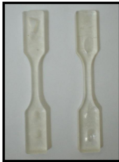
Figure 3.11: Example of Pure Polylactic –acid (PLA) Sample after Injection Molding
