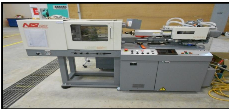
Figure 3.8: Injection Molding Machine (University Malaysia Pahang, Pekan Campus, Mechanical Engineering Faculty)
