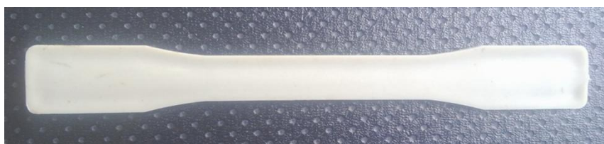
Figure 3.8: Final product of injection moulding for Polypropylene sample
