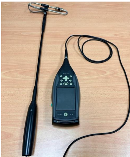
Figure 2. B&K handheld analyzer with sound intensity probe
