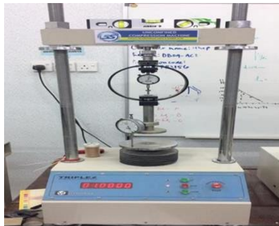
Figure 3. The specimen was compressed under UCT machine.
