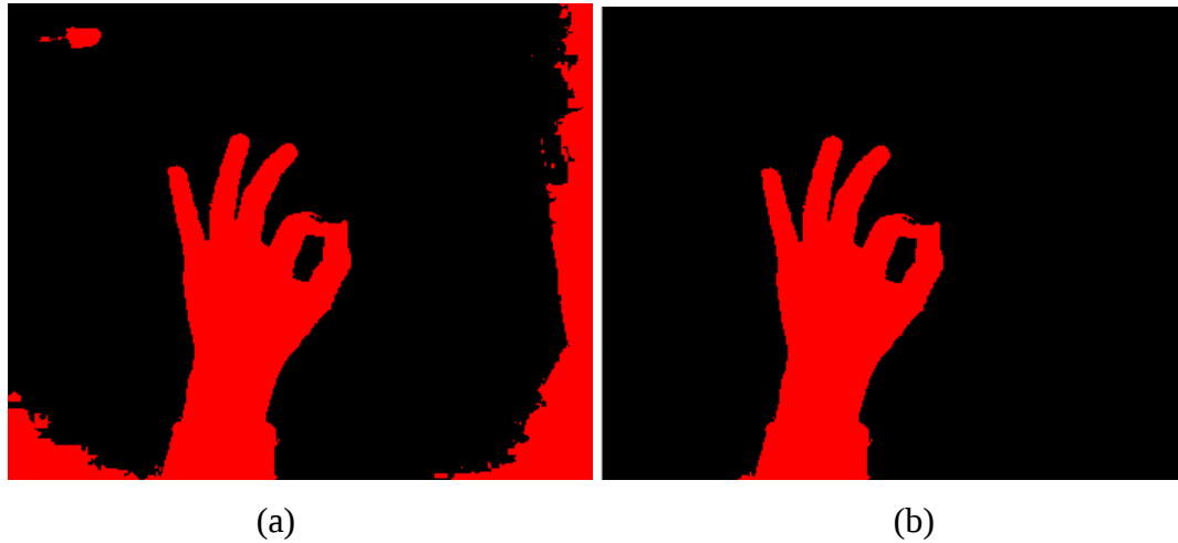
Figure 32: Image Processing Steps (a) Inverse Binary Image (b) Particle Filter
