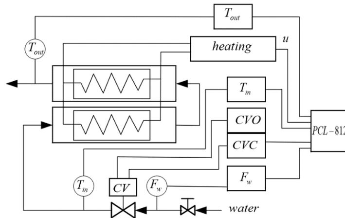
**Fig. 1.** Schematic diagram of electric water heater
