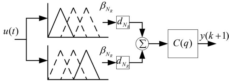
Fig. 5. Fuzzy-Hammerstein structure
