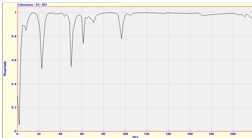
Fig. 11. Graph of coherence for modal testing
