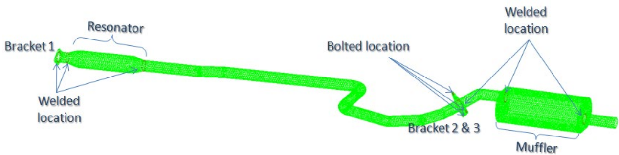
Fig. 1. Exhaust structure FE model mesh in FEA
