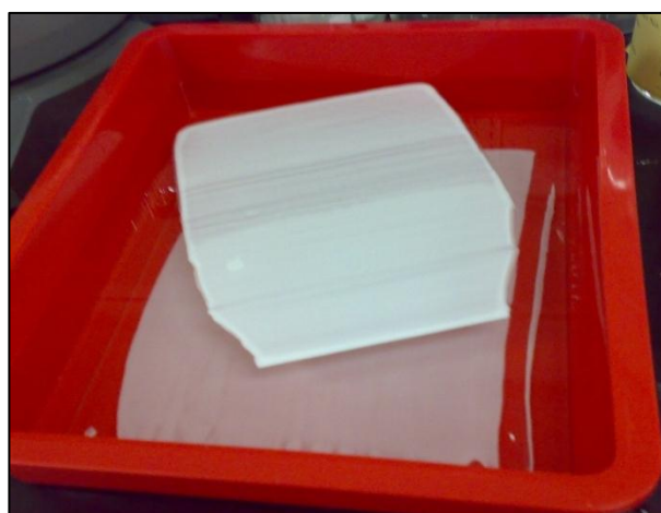
Figure 3.2: Flat sheet membrane formed after immersing in coagulation water bath
