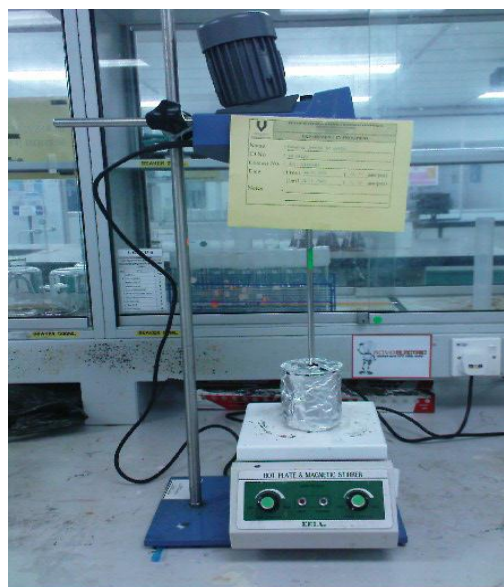
Figure A.6: Equipment used to mixed the resin with membrane polymer to form homogeneous slurry
