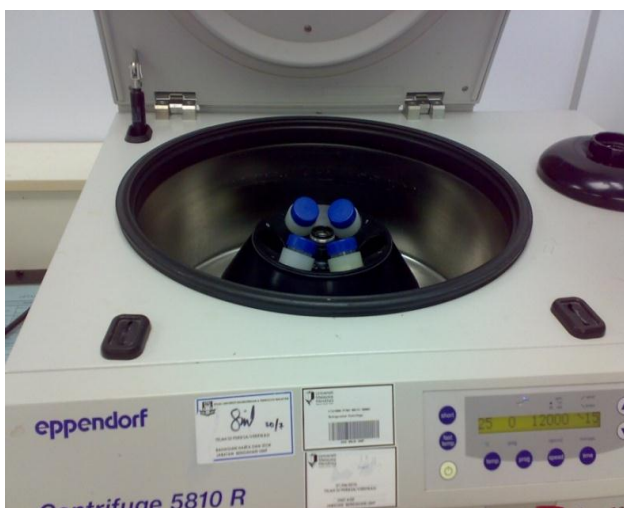
Figure A.5: Equipment used to separate the ground resin from the copper ion solution
