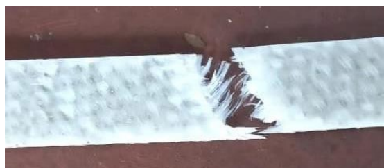
Fig. 2. Failed GFRP specimen
