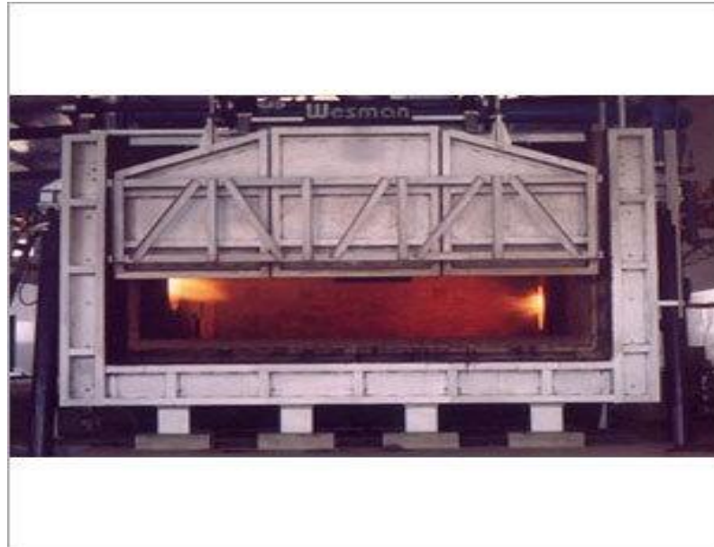
Figure 2.3: Aluminium melting furnace
