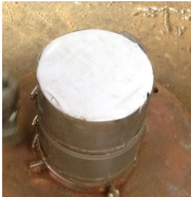
Figure 3.25: Nano size cloth that placed inside the cyclone
