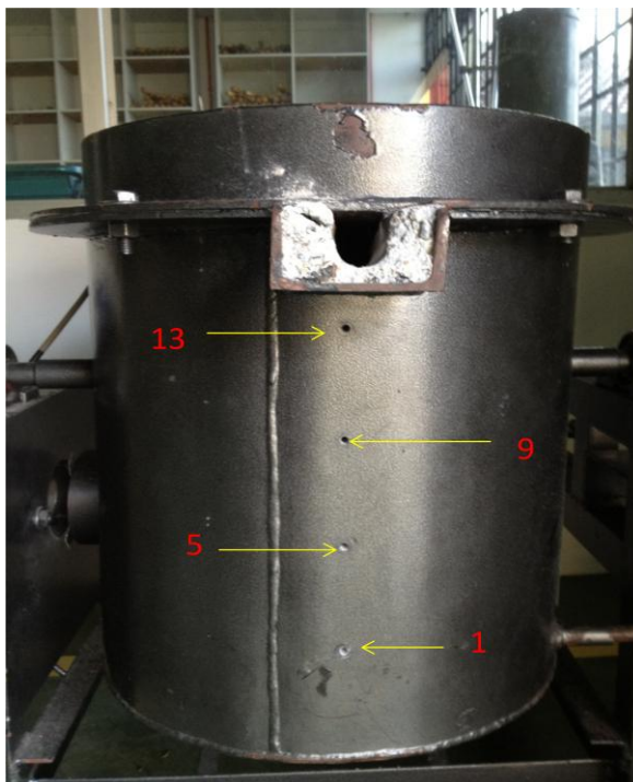
Figure 3.18: Method to place thermocouple
