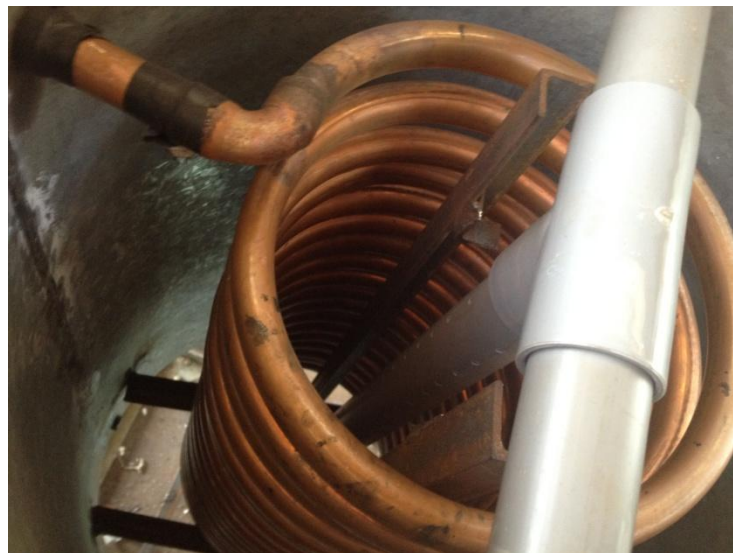
Figure 3.22: A spiral copper coil placed inside the cylinder
