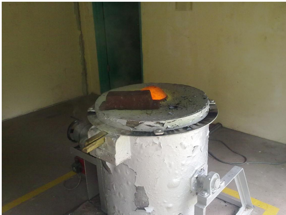
Figure 3.2: Furnace reactor with strainer at the top
