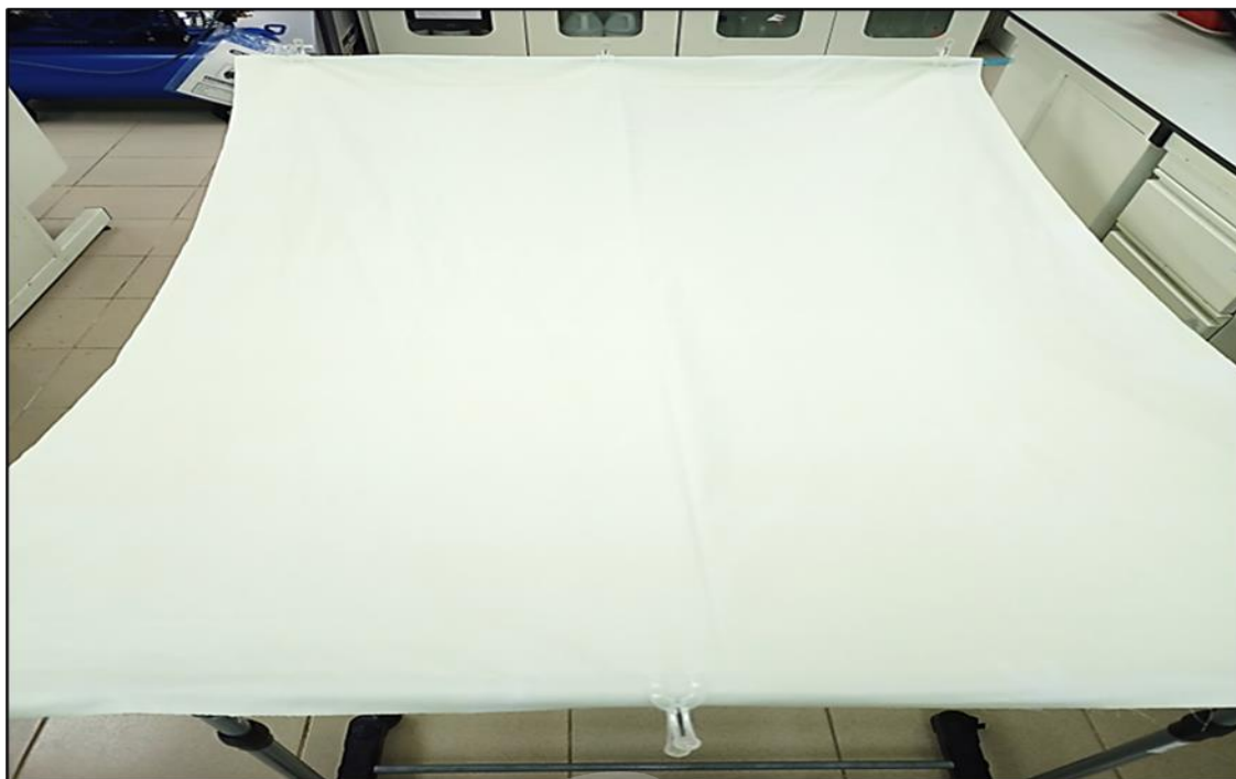
Figure 3.1 Drying method of fabric after the dipping process.
