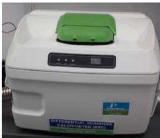
Figure 3.19 Differential Scanning Calorimetry machine (Perkin Elmer DSC8000, USA)
