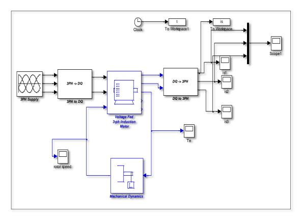
Figure 3.3 Induction Motor Models with Load Using NUDSL
