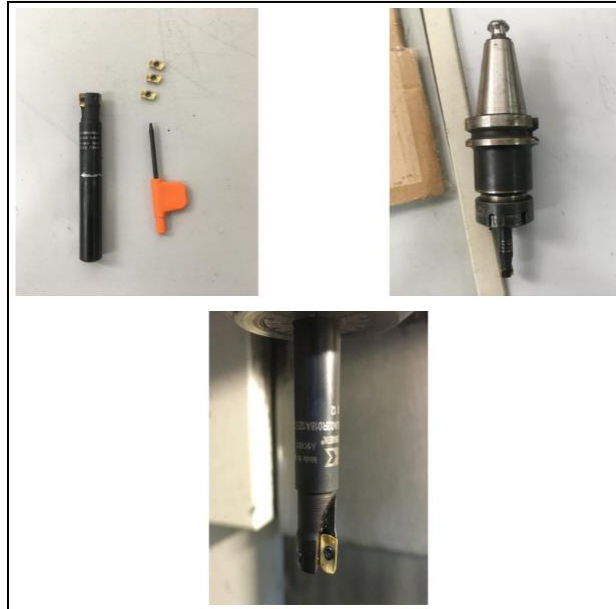
Figure 1: The cutting tool with inserts of coated carbide.
