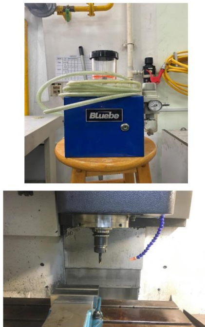
Figure 4: The MQL system and the distance between the nozzle and cutting tool is 100 mm.
