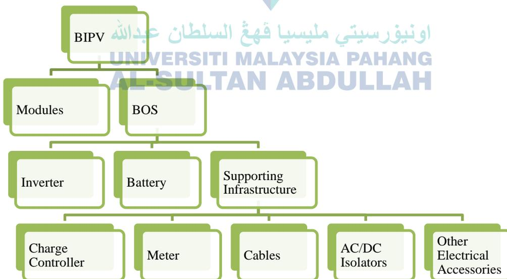
Figure 3.7 BOS Components for BIPV
