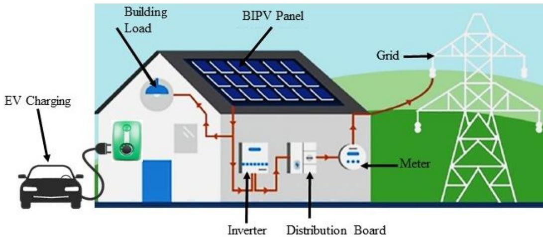
Figure 3.6 Conceptual photograph of solar BIPV + EV system
