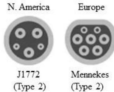
Figure C.2 Type 2 charger's socket
