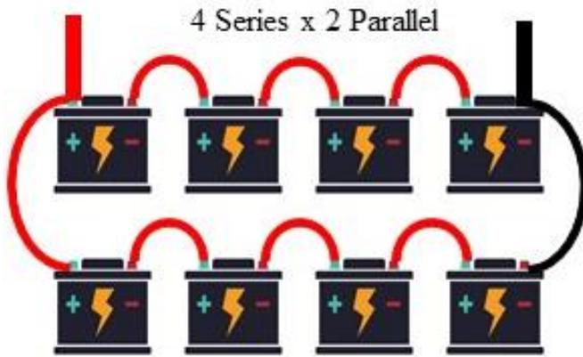
Figure 4.4 Battery layout for Case B
