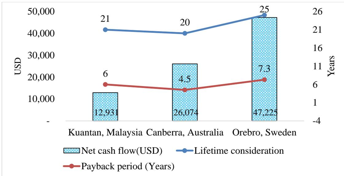
Figure 4.31 Comparison of plant lifetime, payback period and net cash flow
