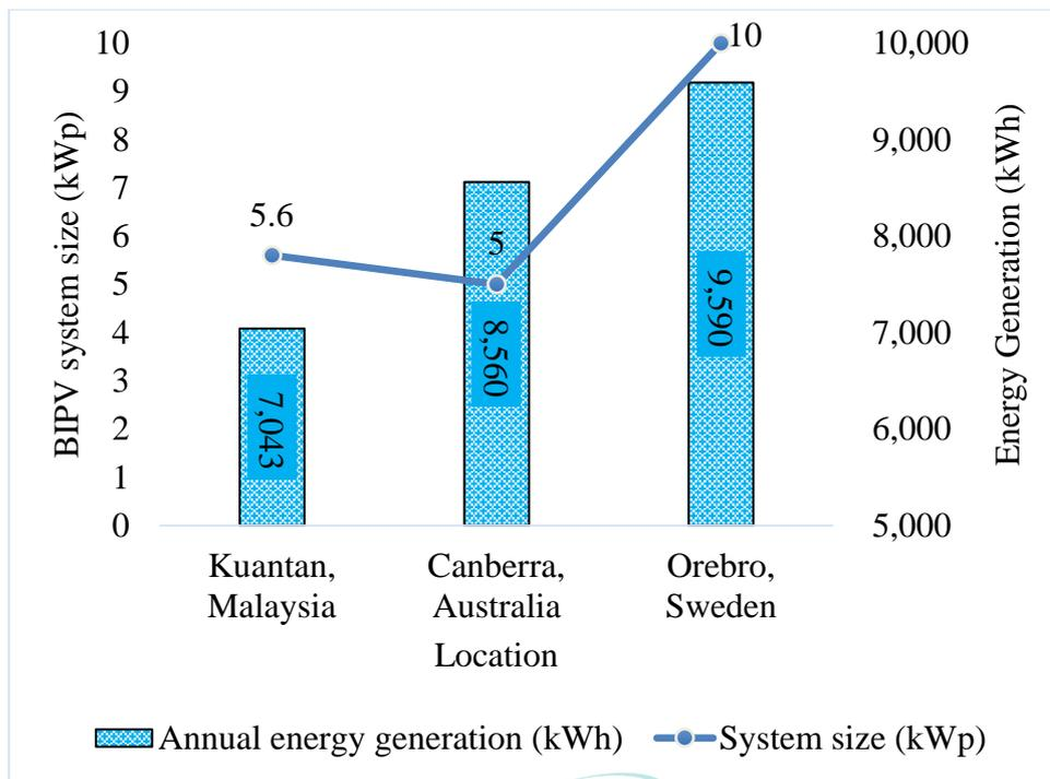
Figure 4.30 Comparison of BIPV system size and annual energy generation in selected location
