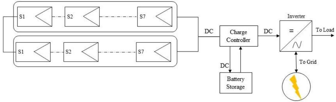
Figure 4.3 Layout of the BIPV system for Case B and Case C
