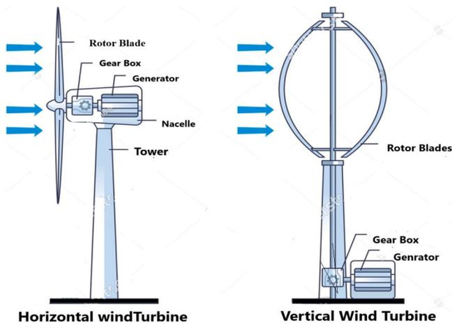
Fig. 3. Comparison between Offshore VAWT and Offshore HAWTs.
