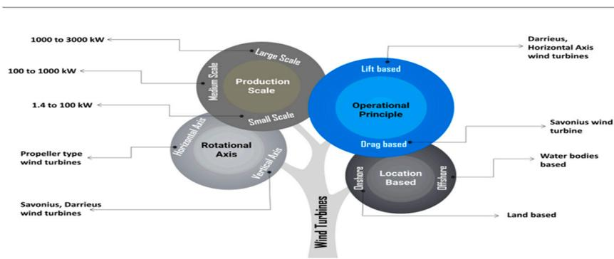
Fig. 2. Wind Tree: A broad classification of wind turbines.
