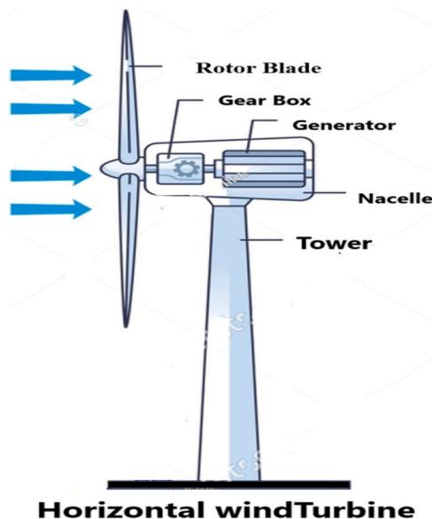
Fig. 5. Small-Scale Wind Turbines Horizontal.
