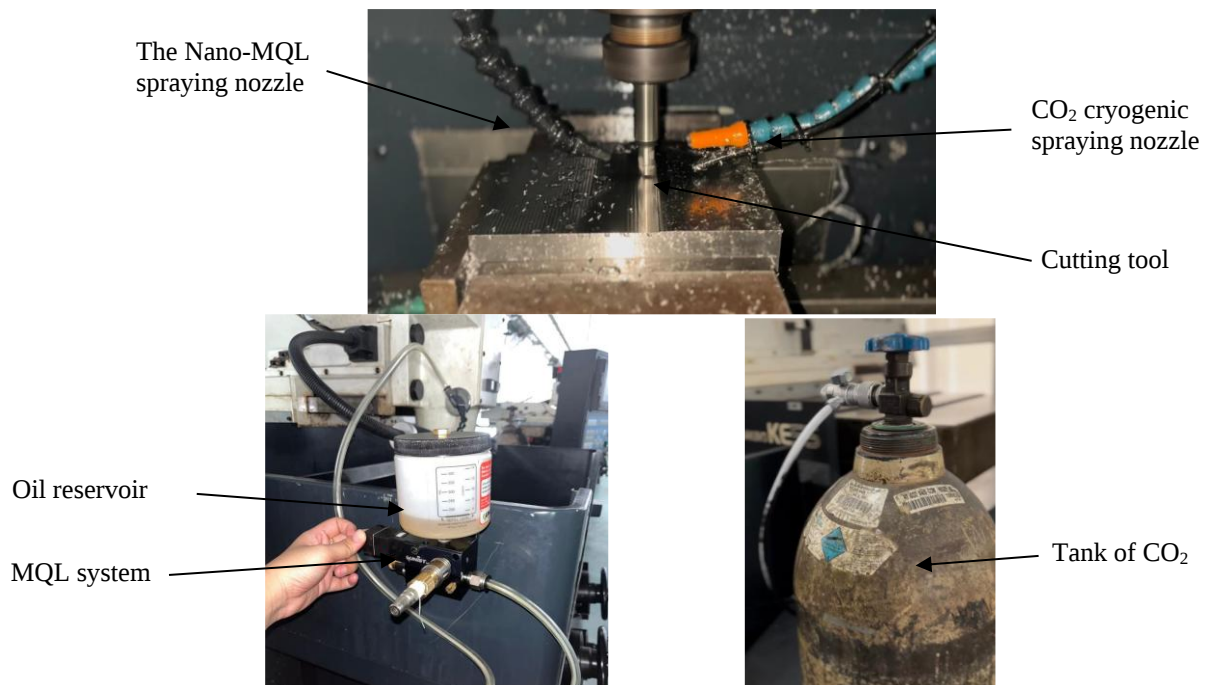
Figure 2: The nano MQL system and the CO 2 cryogenic system set up in milling machine.
