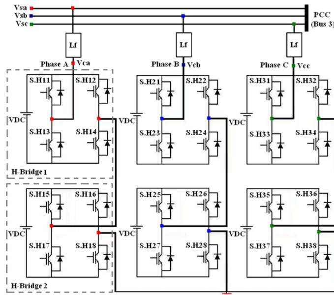
Figure 2. Cascaded H-bridge 5-level VSC
