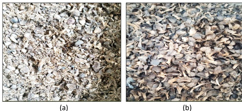
Fig. 2. (a) OPS before processed (b) OPS after processed
