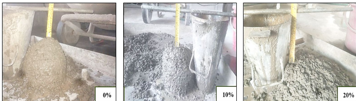
Fig. 5. The effect of CTP content on concrete slump pattern
