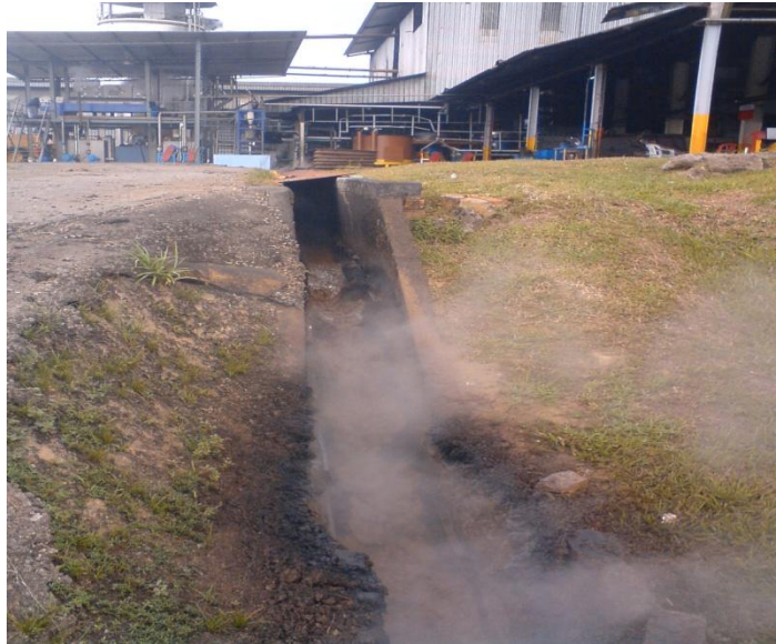
Figure 3.2: Raw POME sampling after the crude palm oil processing
