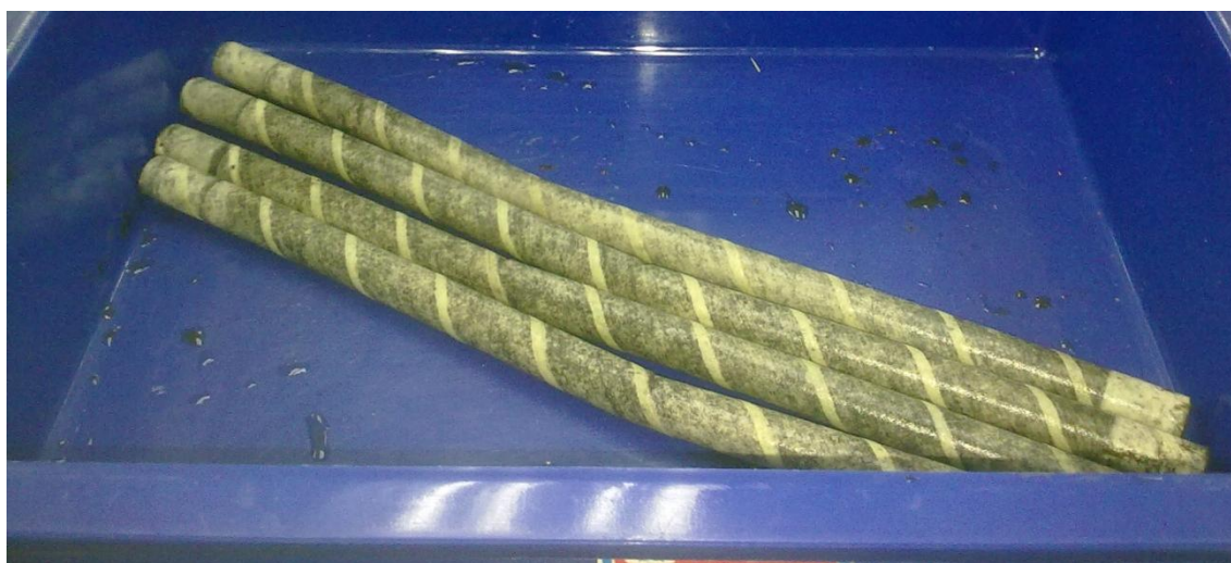
Figure A3.4: Membrane used (before cleaning) during in the cross-flow ultrafiltration (CFU) MAS
